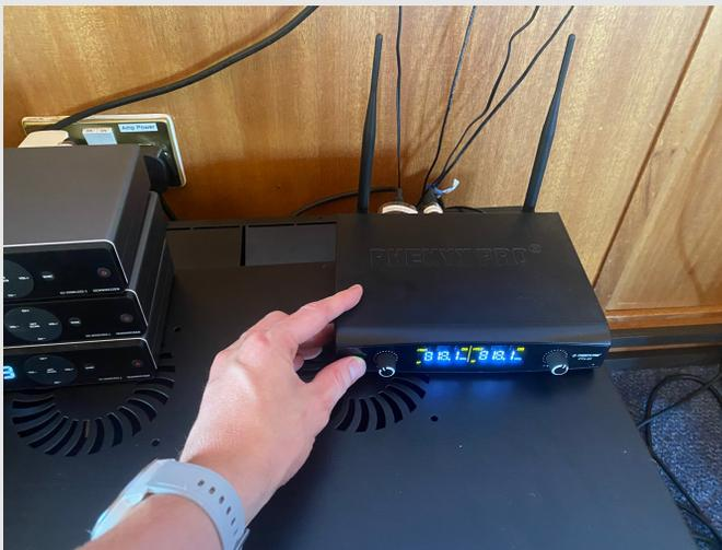
All the Microphones should be on automatically, except the handheld microphones. You need to press the button (as seen on the left, to make them work.
